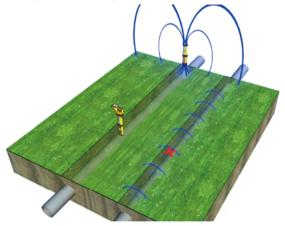
The signal should now only be visible in the wanted service but not on the unwanted service. Note that only one service at a time can be nulled out using this method, so if there are more than two services the above may need to be repeated to null out other services.
