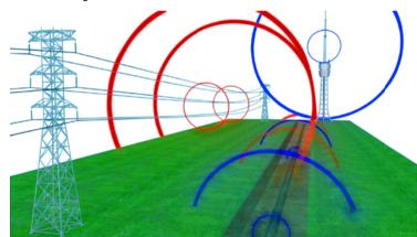
Radio Signals are created by low frequency radio transmitters. These are used for broadcasting and communications. They are positioned throughout the world. As the frequencies are very low the signals tend to penetrate and hug the curvature of the earth. When the signals cross a long conductor such as a pipe or cable, the signals are re-radiated. It is these re-radiated signals that can be detected by the Radio Mode.
