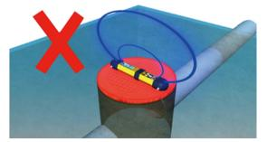
When using the Induction mode, avoid placing the transmitter over metallic manhole covers as this will severely reduce the effectiveness of the transmitter and in extreme cases cause damage to the transmitter's circuitry.
