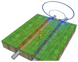
2. Now position the vScan receiver exactly over the unwanted signal. The person at the transmitter end can now hold the transmitter vertically over the position of the unwanted signal. Move the transmitter side to side across the line of the unwanted service whilst asking the person at the receiver end to indicate when the signal is "nulled out". Insert the transmitter into the Tx foot and place in the null position.
