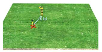
Position the vScan receiver approximately 10m from the transmitter and with the flat of the blade pointing directly at the transmitter. Switch it on and adjust the sensitivity so that approximately 20% reading is observed.
