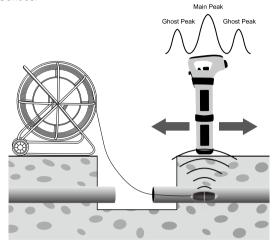
5. Now sweep left and right over the Sonde to obtain a second peak. Note that there are no ghost signals when sweeping left to right over the Sonde.
